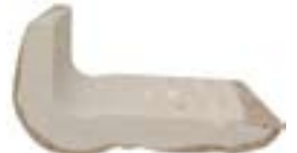
This is an acceptable profile of an irregular back tile.
