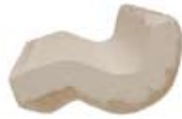
This is an acceptable profile of an irregular backed tile.
